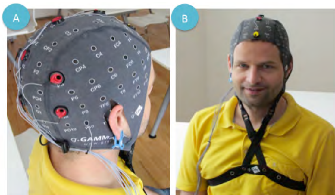
Figure 6: The cap is positioned such that the Cz electrode...
