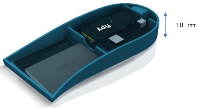
Figure 17 - 3D Model of Pycom Insole Hardware Housing Layout
