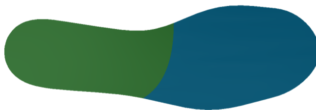
Figure 12 - Insole Usable Area (green: rigid, blue: flexible)
